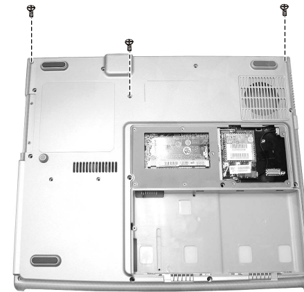
Figure 2-26 Remove the metal shield
