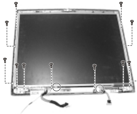
Figure 2-22 Remove LCD panel
